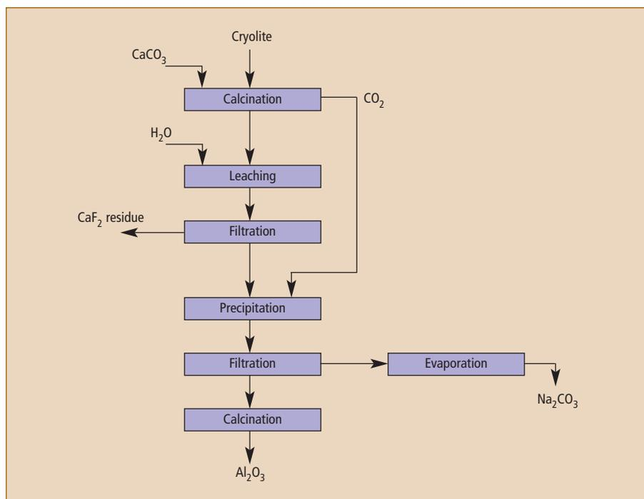
Fig. 13. Thomsen's process for the recovery of  $\text{Al}_2\text{O}_3$  and  $\text{Na}_2\text{CO}_3$  from cryolite.
