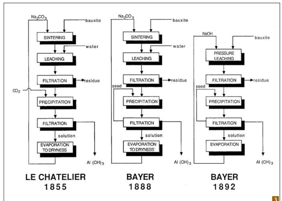
Fig. 3. The shift from the thermal route (Le Chatelier process) to the hydrometallurgical route (Bayer process) for the production of alumina.
